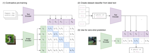
Figure 1. Summary of our approach. While standard image models jointly train an image feature extractor and a linear classifier to predict some label, CLIP jointly trains an image encoder and a text encoder to predict the correct pairings of a batch of (image, text) training examples. At test time the learned text encoder synthesizes a zero-shot linear classifier by embedding the names or descriptions of the target dataset’s classes.
