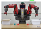
(i) A Baxter performing a sorting task synthesized from natural language. Boteanu et al. (22)
