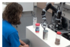
c) A Jaco arm identifying objects from attributes, here "silver, round, and empty." Thomason et al. (173)
