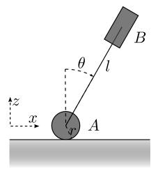
Consider an inverted pendulum mounted on a wheel in the 2D x-z-plane; similar to a Segway. The exercise is to derive the Euler-Lagrange equation for this system.
